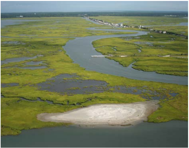
MARSH RESTORATION In Avalon, NJ, thin layer placement of sediment across low-lying and degraded sections of the salt marsh helped restore native plants to keep pace with sea level rise (Image Credit: TNC)
