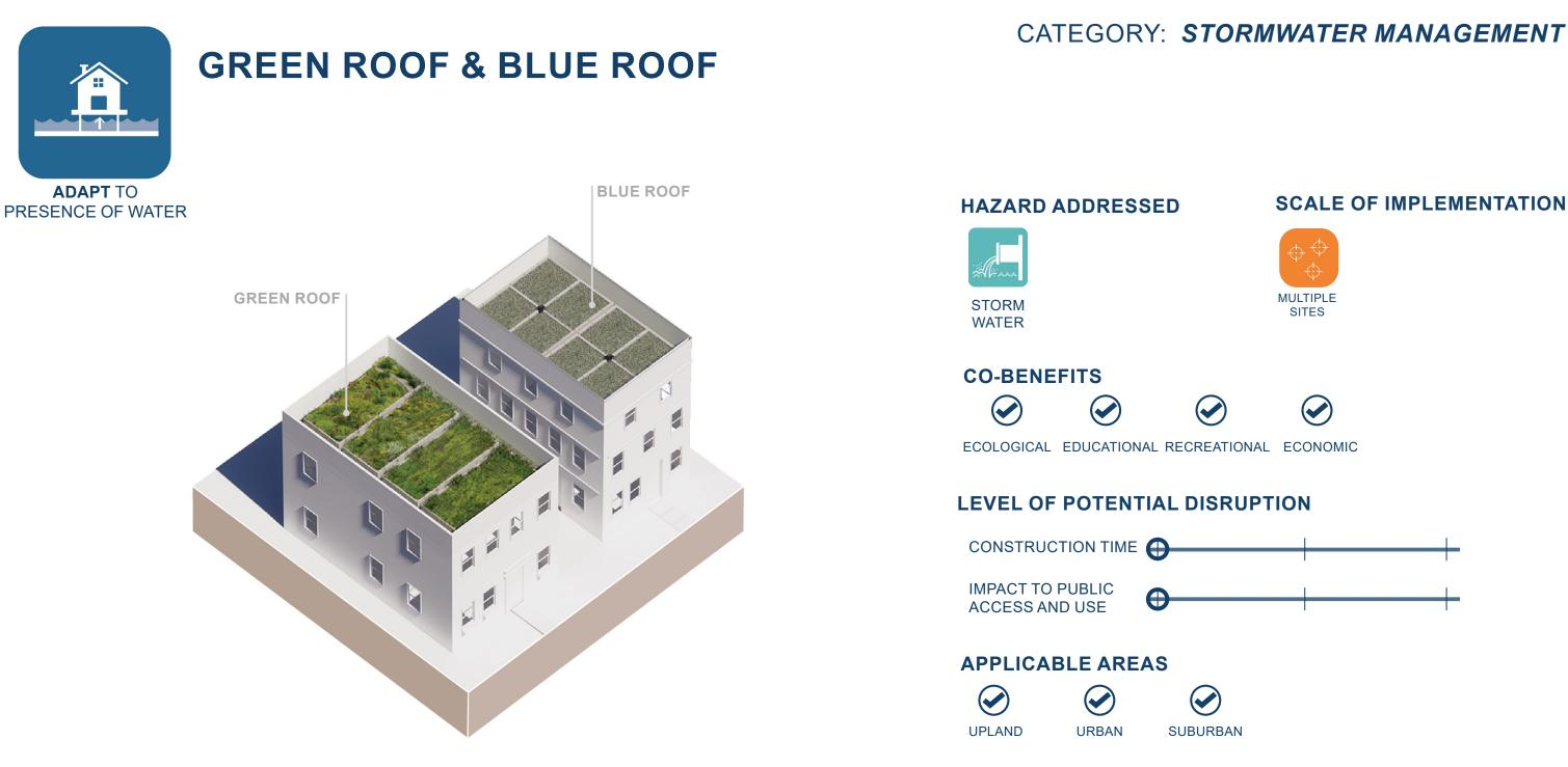
A green roof is a layer of growing medium for vegetation installed over a waterproofing system, slowing down runoff by retaining rainwater and gradually COSTS releasing it back into the atmosphere through condensation and transpiration. Blue PERMITTING roofs provide temporary water storage systems that allow for the gradual release or evaporation of stored water.
